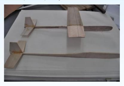
5 .Check that the parts of the aircraft are glued together in a straight line and
